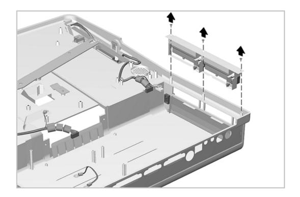
Figure 7-26. Removing the PC Card Door Assembly Reverse the above procedure to install the PC Card door assembly.
